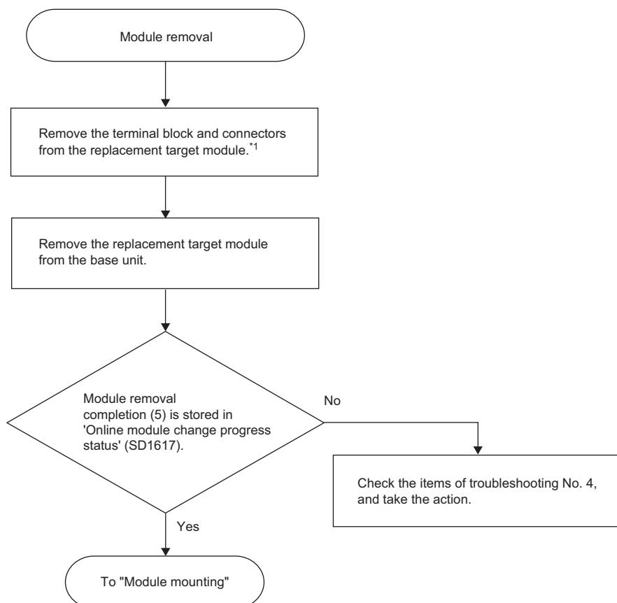
\*1 Remove the SD memory card from the module to be replaced when MES interface module, high speed data logger module, C intelligent function module, and OPC UA server module are used.
