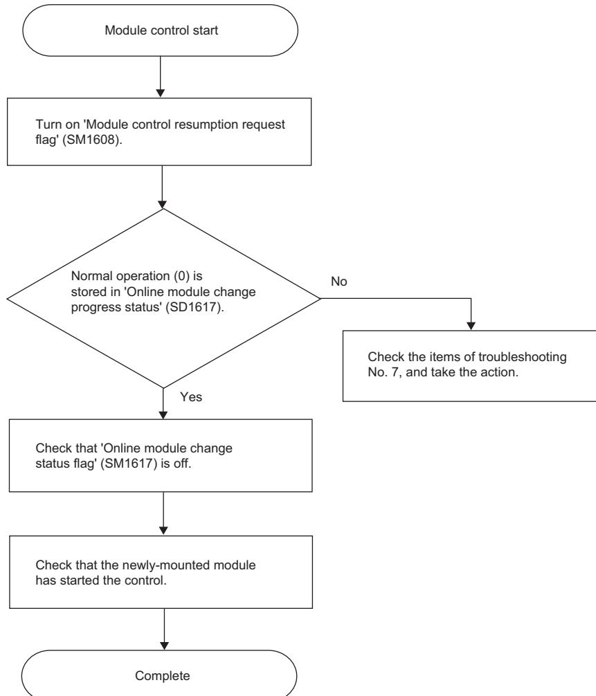
To check the control restart, check the following depending on the module.
